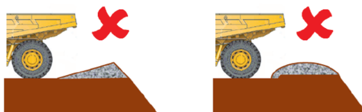
UNSUITABLE EDGE PROTECTION BERM PROFILE
