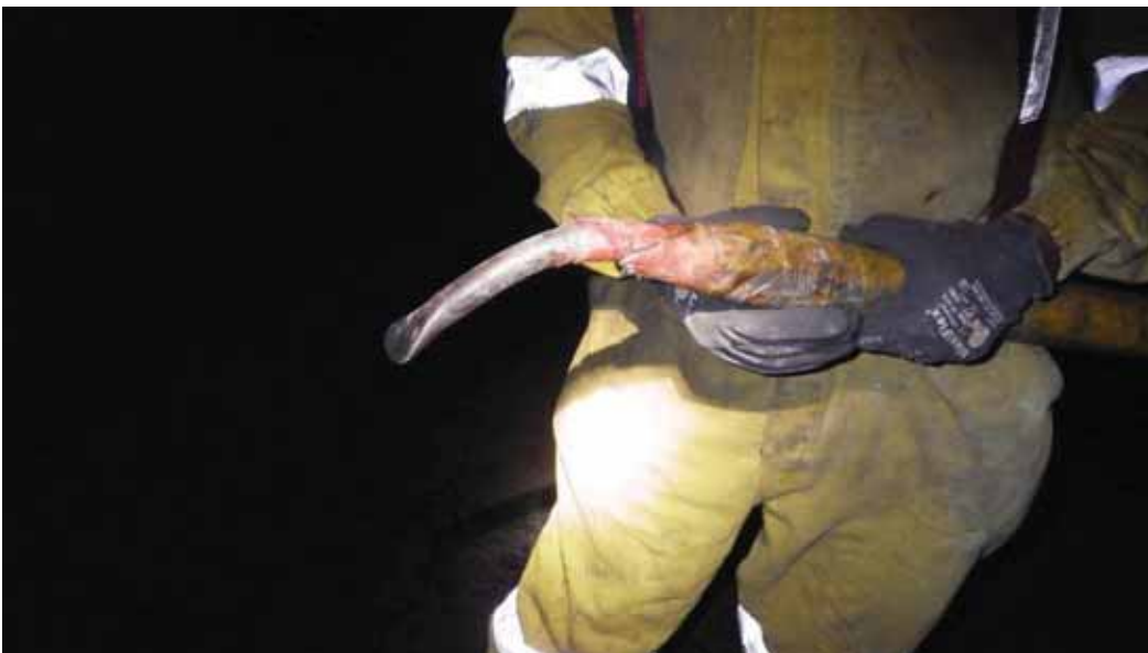
Figure 36: Fibre-glass combination pinch bar with sounding stick on one side and pinch bar on the other (Mining House G)
