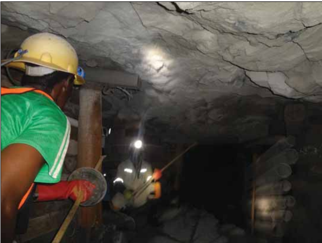
Figure 59: Pinch bars being used with and without hand guards/ gaskets at Mine 8
