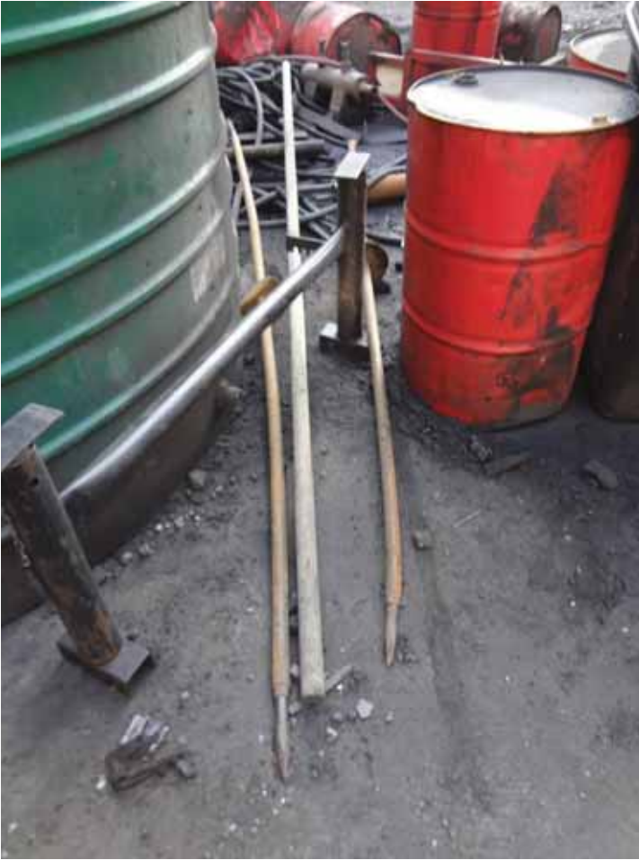
Figure 41: Discarded old and bent pinch bars on surface (Mine/ Shaft 3)
