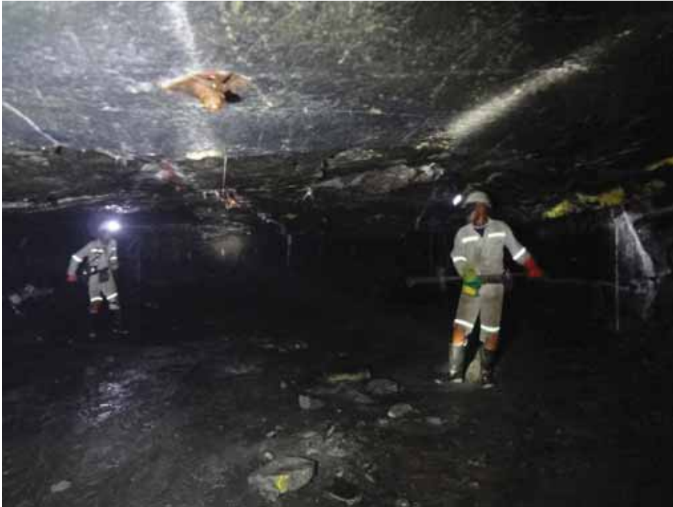
Figure 187: Example of extent of illumination with the use of the EE light (No flash was used on portable camera)
