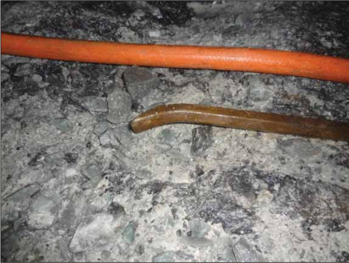
Figure 58: Worn/ Old pinch bar with blunt end (Mine 1)
