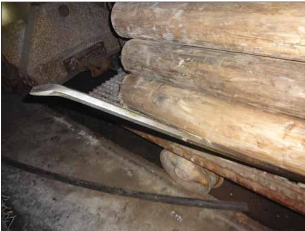
Figure 22: Incorrect usage of pinch bar for a task not intended for the equipment (Mine 11)
