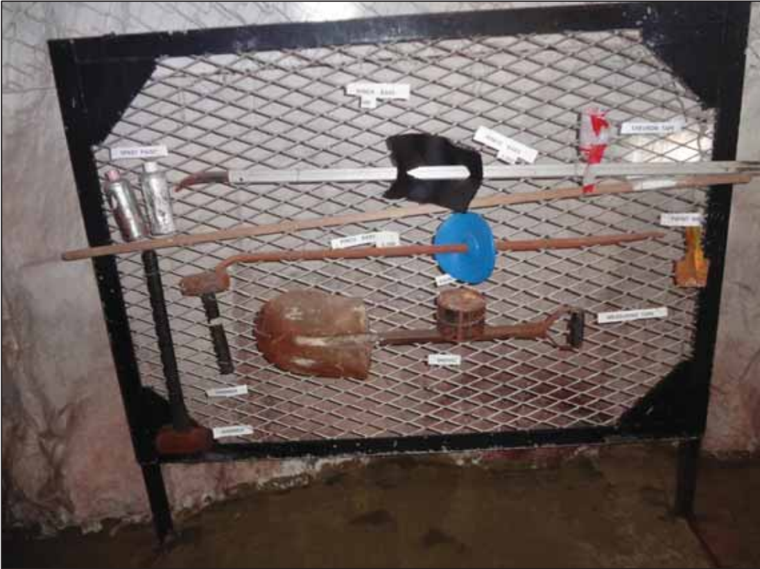
Figure 17: Typical entry examination board displaying the tools needed to bar (Mining House C)
