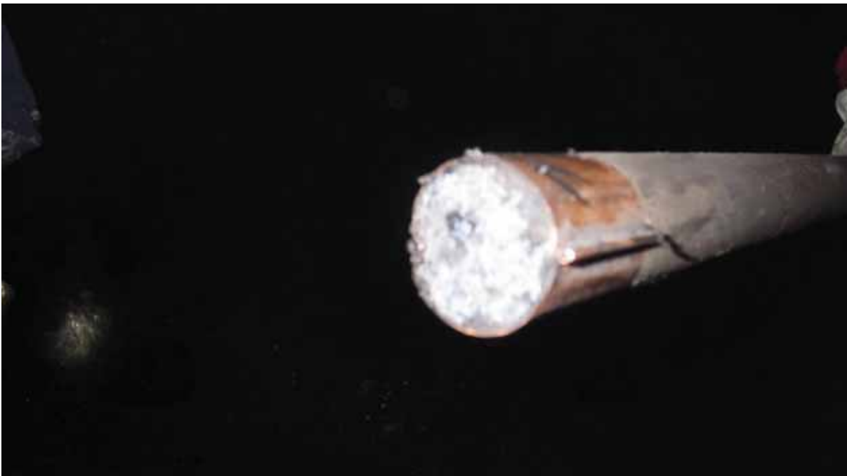
Figure 38: Traditional wooden sounding stick with copper end – Note that the copper end does not cover the flat end of the stick. Suppliers are currently being contacted to ascertain the reasons for this – Mining House H.
