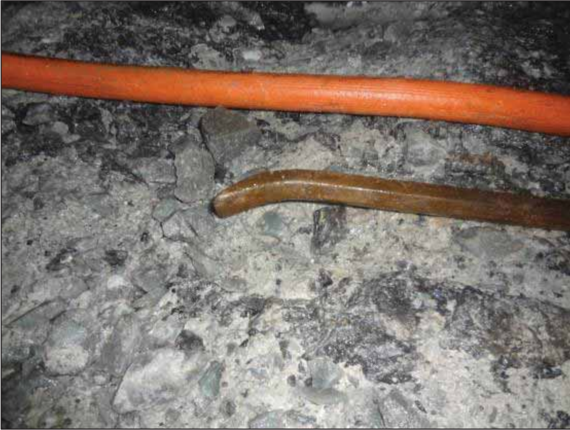
Figure 66: Worn/ Old pinch bar with blunt end (Mine 1)
