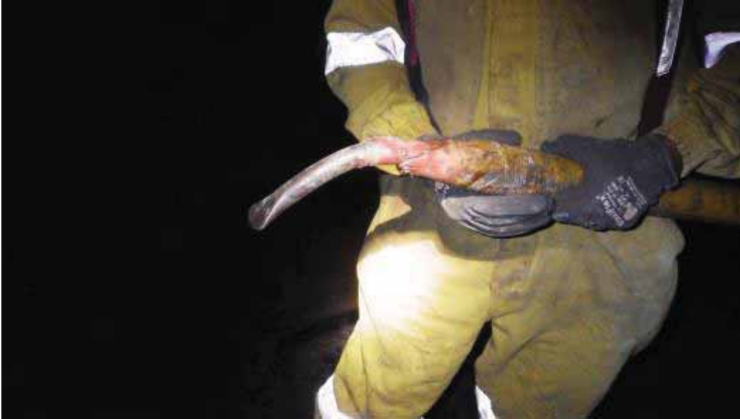
Figure 48: Fibre-glass combination pinch bar with sounding stick on one end and pinch bar on the other (Mining House G)
