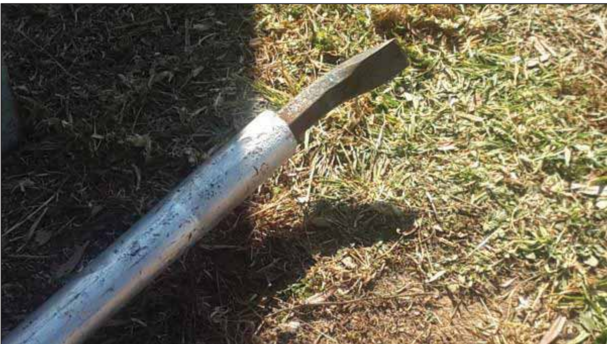
Figure 69: 3m long Aluminium pinch bar used at a mock mine (Mine 12)
