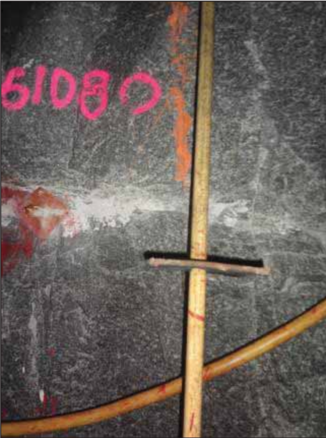
Figure 36: 3m long Fiberglass pinch bar with conveyor belt gasket used at a development end at Mine 8. This gasket is sturdy enough to deflect rock fragments but is hard to move up or down the pinch bar. Note also that the bar is not located in the middle of the gasket.
