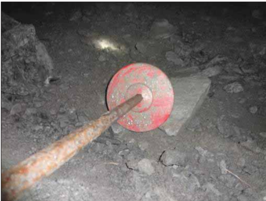
Figure 33: Incorrect usage of a drill steel gasket which does not fit tightly onto the pinch bar (Mine 6)
