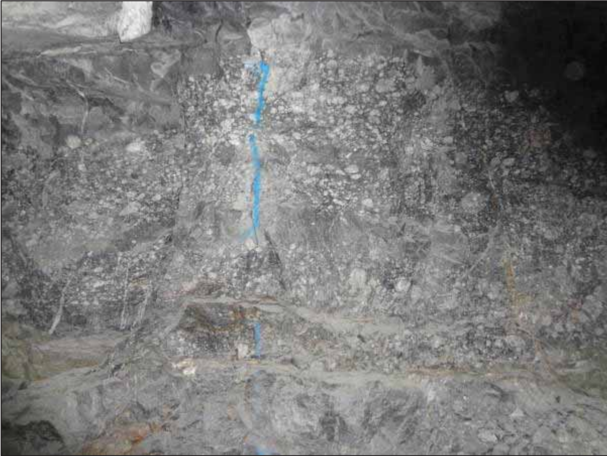
Figure 73: Minor faulting in VCR (Mining House D)
