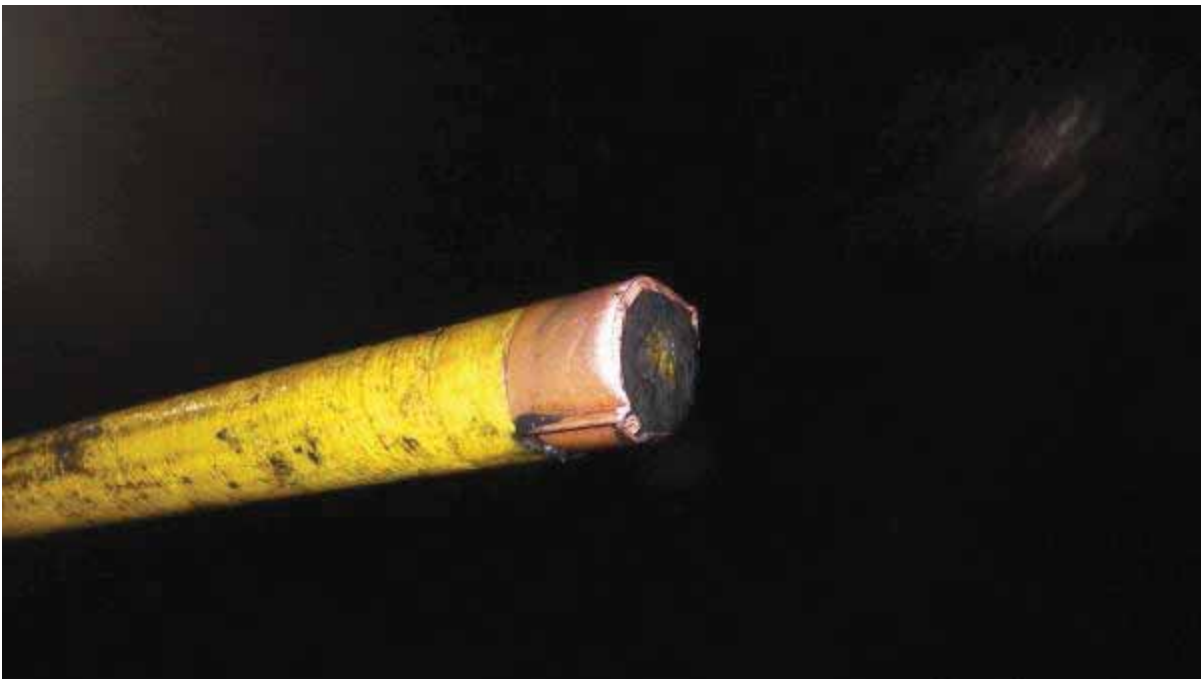
Figure 49: Opposite end of fibre-glass pinch bar i.e. sounding stick side with copper end (Mine/ Shaft 7)
