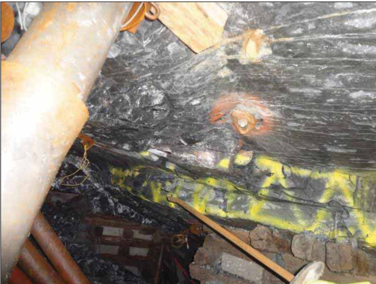
Figure 71: Layering and stress-induced fractures in lava hanging wall (Mine 8)
