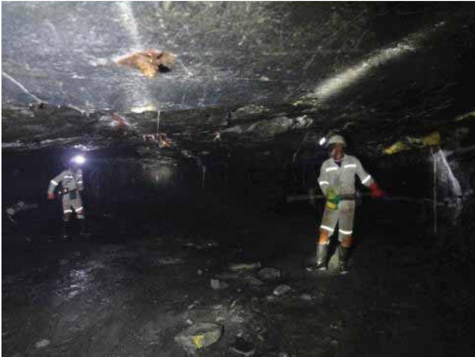
Figure 195: Example of extent of illumination with the use of the EE light (No flash was used on portable camera)
