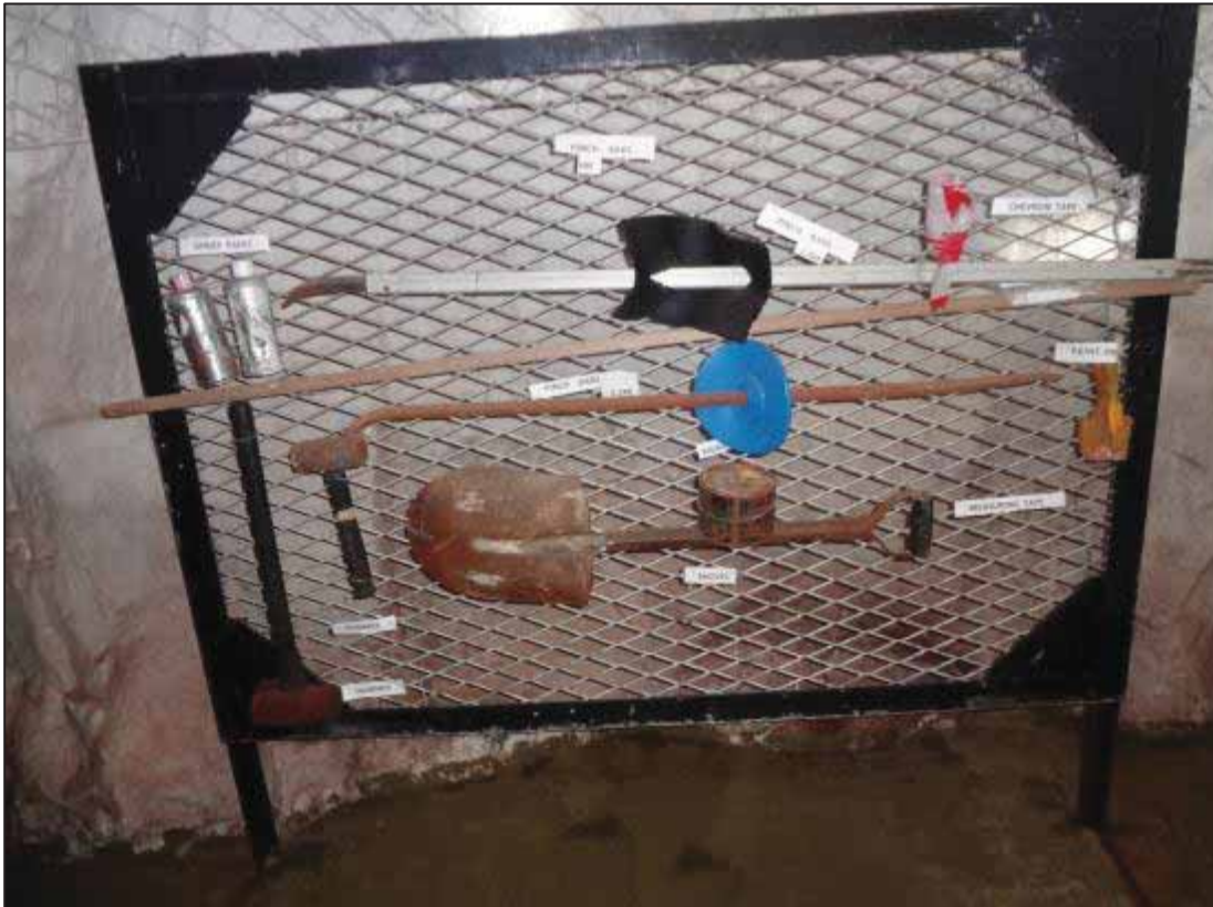
Figure 32: Typical entry examination board displaying the tools needed to bar (Mining House C)
