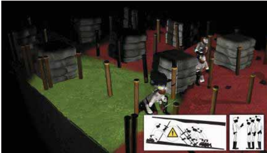
Figure 207: Characters in the lesson plan shown in-stope (red area indicating the no-go zone)
