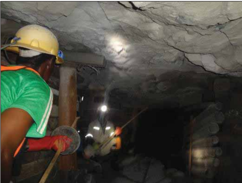
Figure 67: Pinch bars being used with (good practice) and without (poor practice) hand guards/ gaskets at Mine
