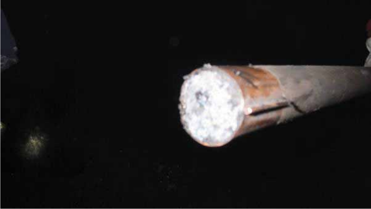
Figure 50: Traditional wooden sounding stick with copper end – Note that the copper end does not cover the flat end of the stick – Mining House H.
