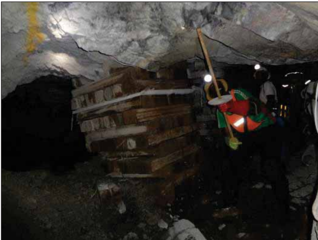
Figure 75: Typical conventional gold mine stope where height of excavation is less than 2m (Mine 8)
