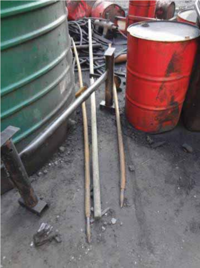
Figure 52: Discarded old and bent pinch bars on surface (Mine/ Shaft 3)
