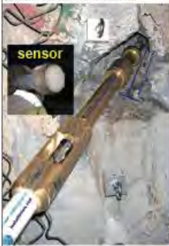
(a) Bottom-view sonde under installation
