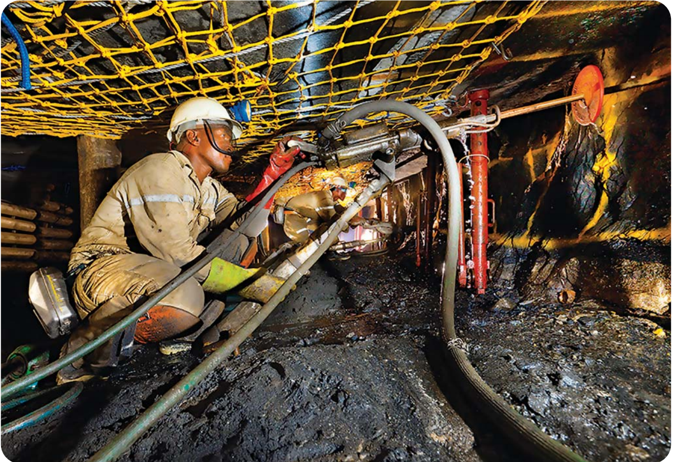
Figure 13. Drilling at right angles to a well-marked face, with top and bottom contact lines and drilling direction lines indicated. The angle of the drill is close to parallel to the top contact
