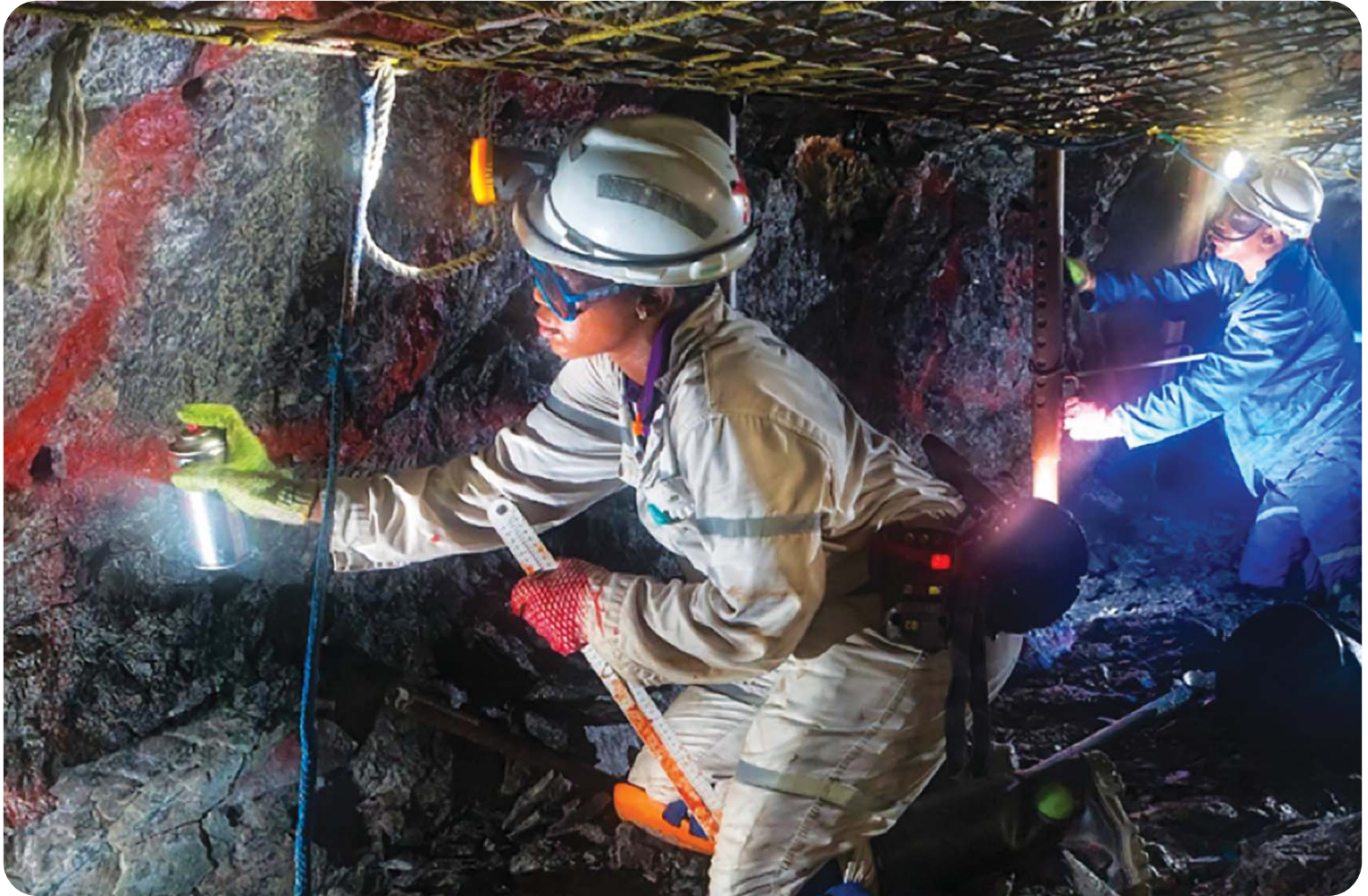
Figure 11. Accurate, clear marking of the face to indicate where the shot-holes should be drilled is critical to executing a good blast
