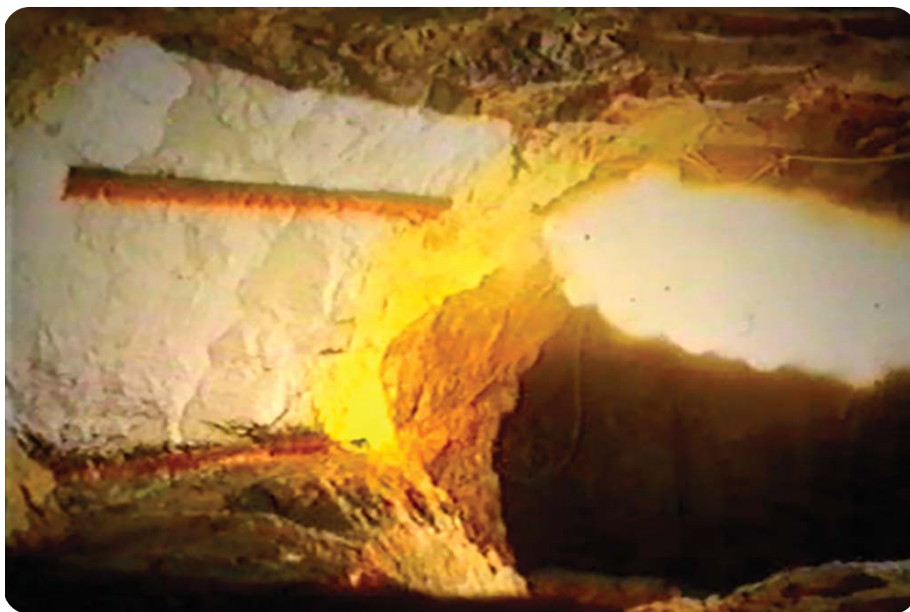
Figure 16. Energy blow-out from blast hole as a result of a lack of stemming (COMRO, 1990)
