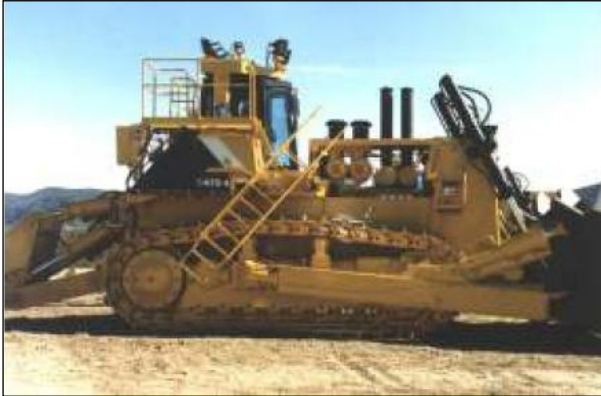
Figure 8: Ladder being rotated to storage position
