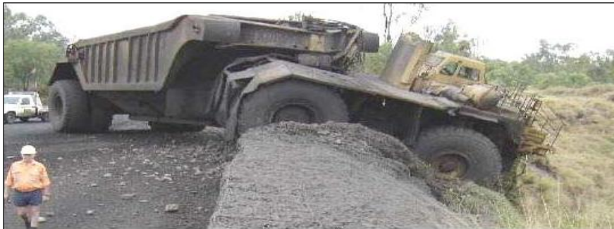
Figure 19: Berm construction material too yielding
