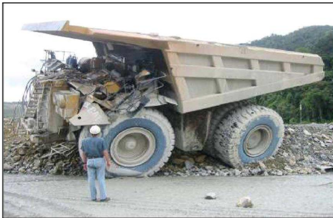
Figure 12: The cab of a truck is crushed by running into the tray of another truck
