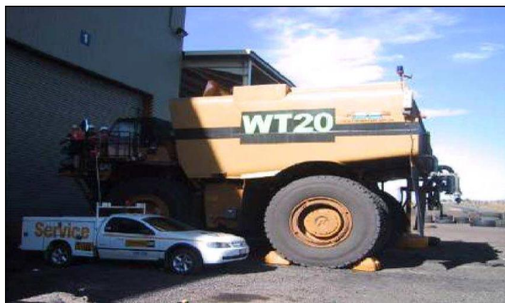
Figure 13: Correct placement of chocks
