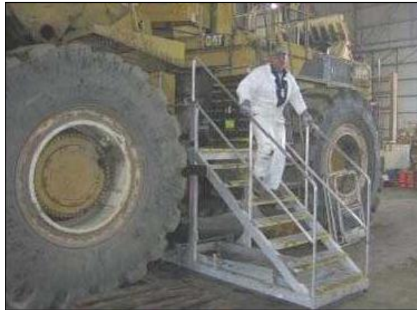
Figure 6: Mobile work platform
