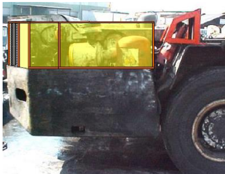
Figure 2: Engine noise hood side view R.H. side opposite driver (25).
