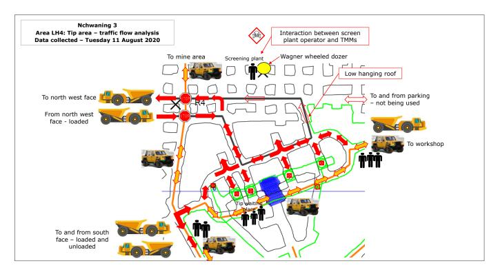
The analysis led to improved illumination at intersections and main haul road through the installation LED lights across the entire mine. The separation of the mine into various geolocations resulted in dedicated signages at various points which allowed for better directed traffic movement. Roadway maintenance has also become a priority during operational planning sessions.
