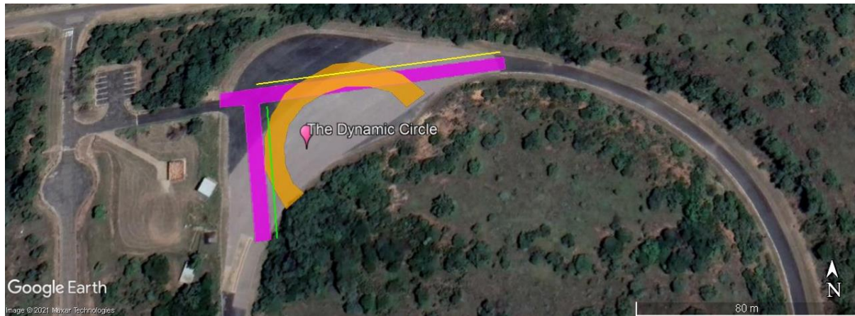
Figure 9: Intersection test on the Dynamic Circle, approximately 100m run-up from the east (yellow line) and 50m run-up from the south (green line), 35m radius curve test in orange
