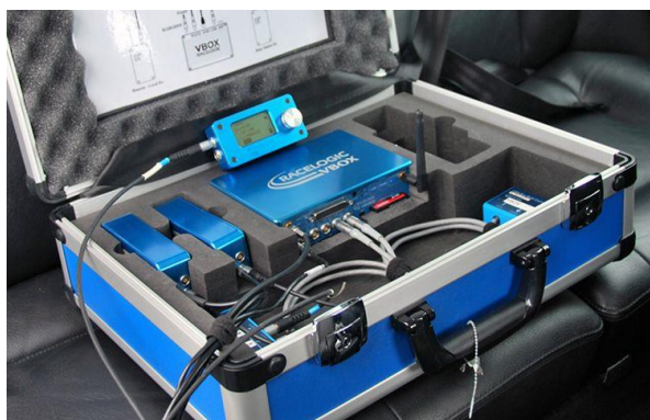
Figure 4: Racelogic VBOX VB3i differential GNSS with dual antenna and IMU (left); VBOX Sigma (right)
