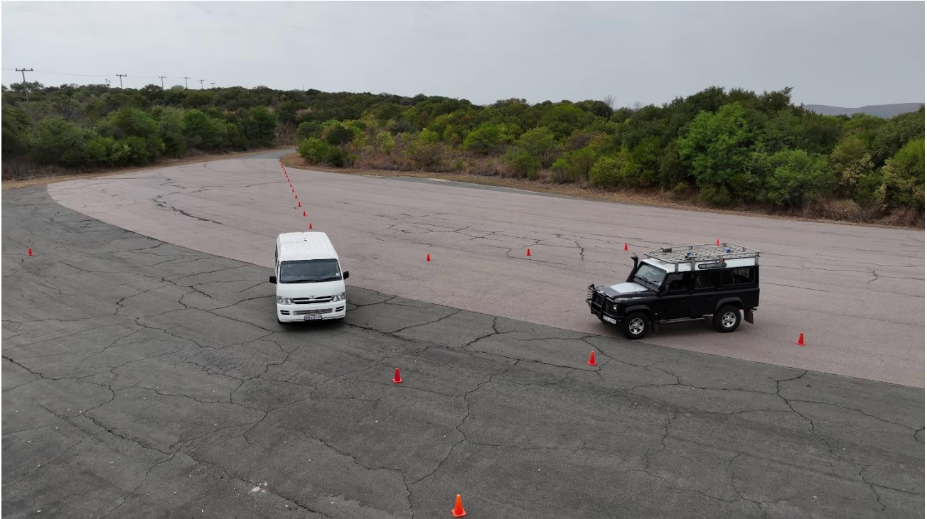
Figure 10: TRL4 CxD Surface Interaction Scenario Test – Test configuration 6: T-junction
