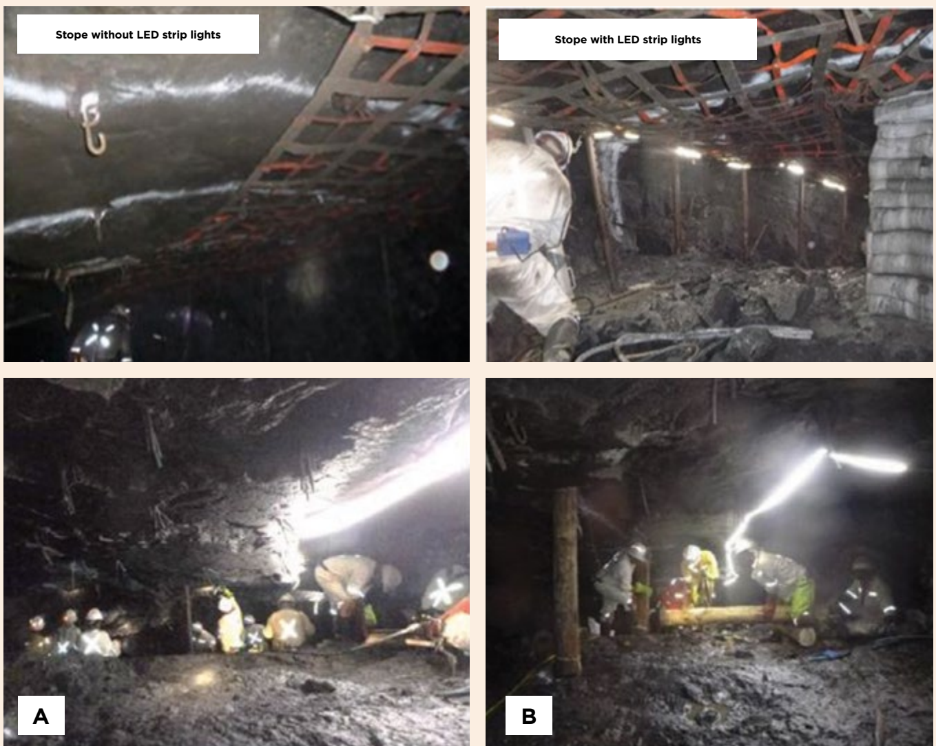
Figure 8: Demonstration of effectiveness of LED strip lights in a conventional stope at Dishaba mine
