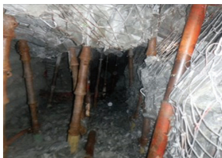
Undercut panels with stoping width 1.8m – RB80 props and steel netting
