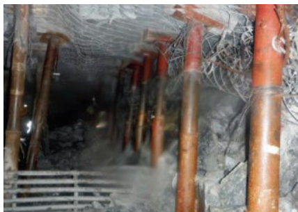
Open cut panels with stoping width >2.5m – Omni props and steel netting
