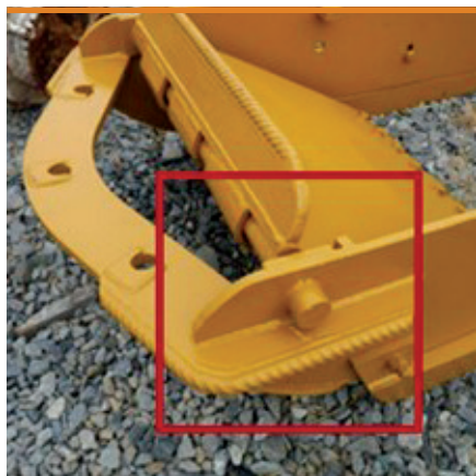
Changes made to the scraper and drilling machine to install netting in low stoping widths.
