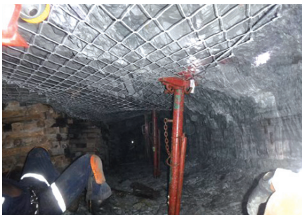
In-stope permanent netting installed with rock-studs and temporary mechanical jacks in a panel at Masimong Mine.
