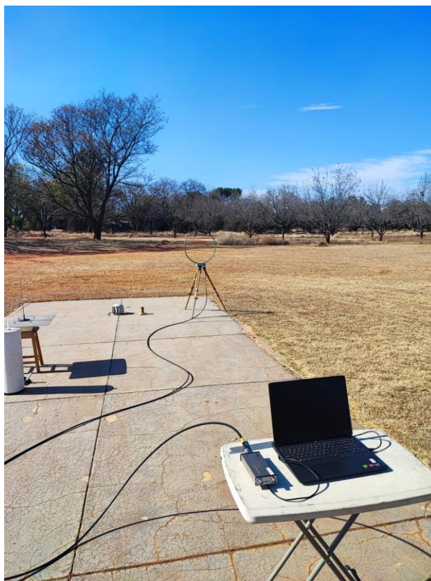
Picture 3: Loop Antenna (10kHz to 1MHz) Setup
