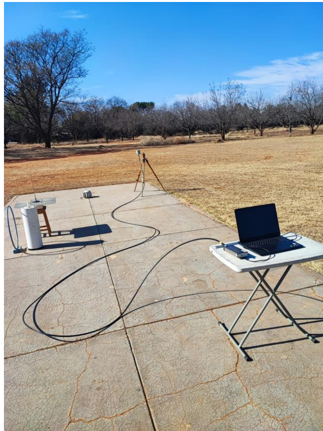
Picture 5: Omni Antenna (1GHz to 6GHz) Setup
