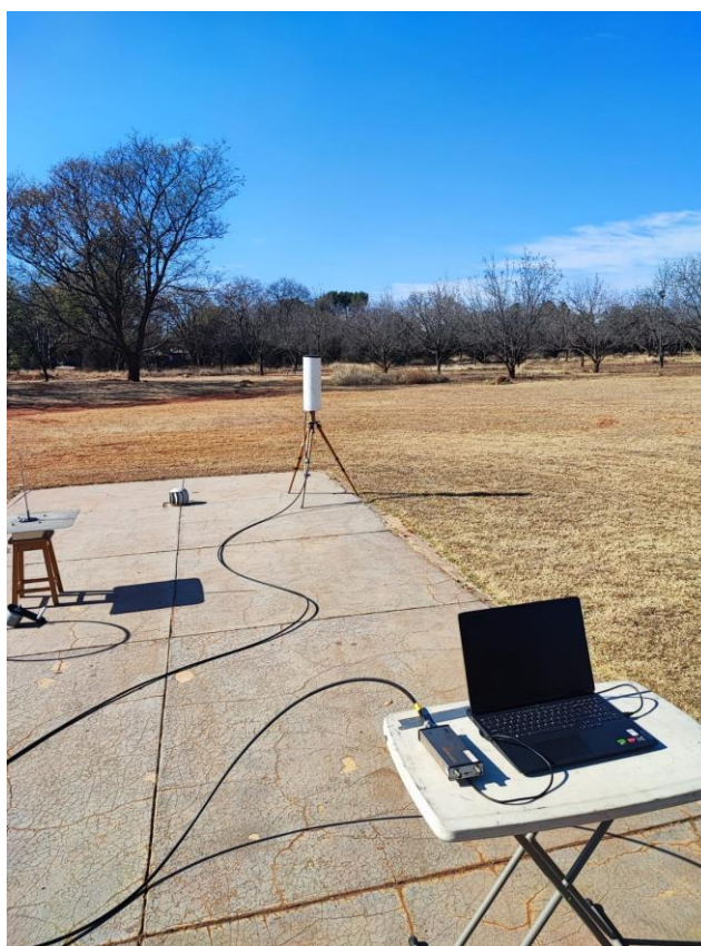
Picture 4: Omni Antenna (100MHz to 1GHz) Setup
