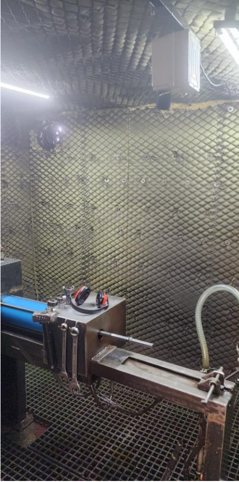
Rockdrill test bench
