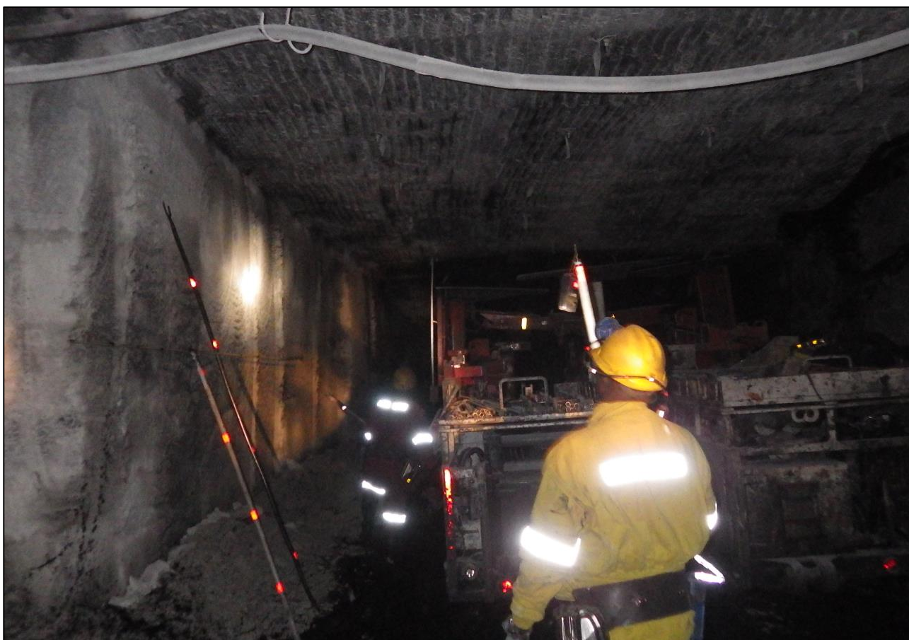
Figure 48: Equipment made more visible with the addition of reflective tape on pinch bars and sounding sticks
