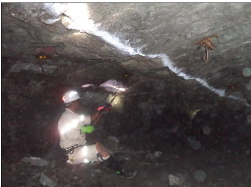
Figure 65: Incorrect stance- positioning and footing. Kneeling would have been preferred to sitting
