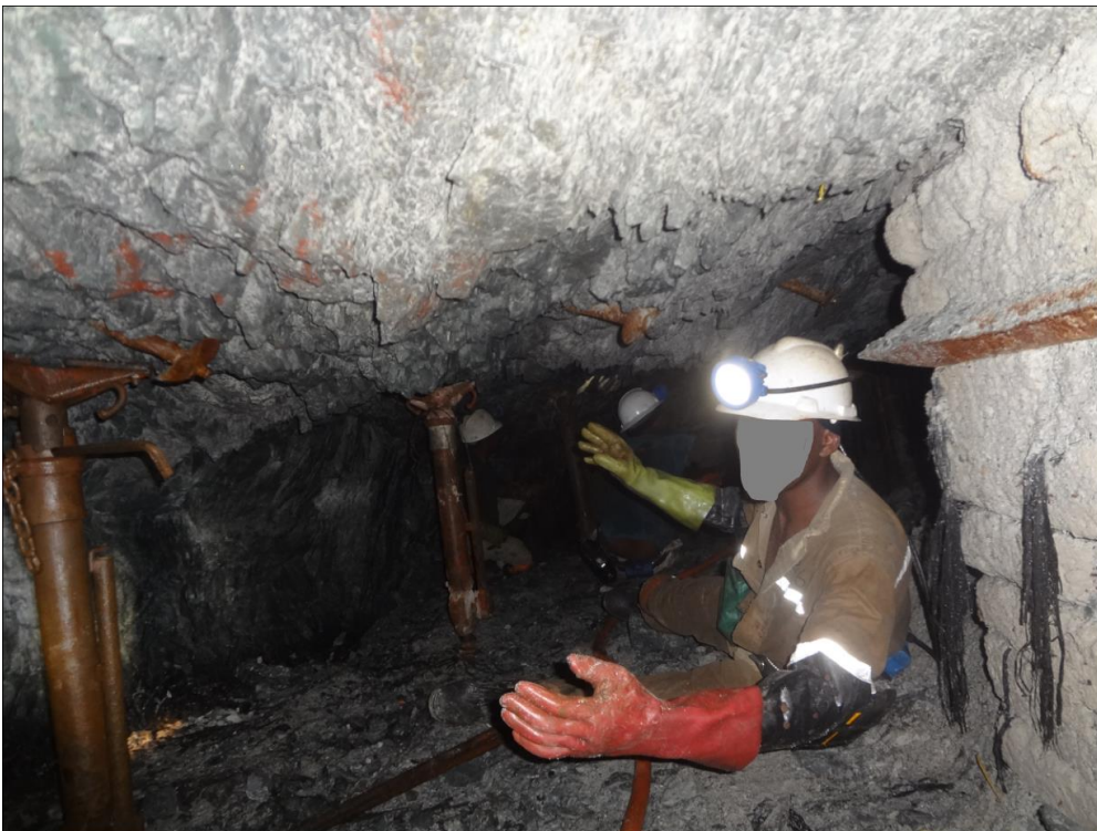
Figure 24: Confinement in-stope due to accumulations of ore
