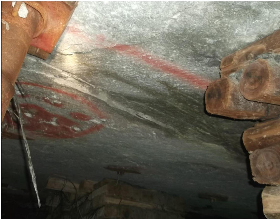
Figure 90: Good Quartzite HW conditions in the back area
