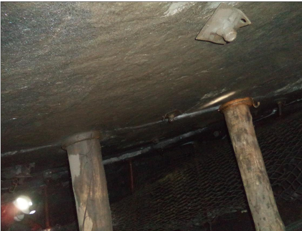
Figure 67: Good Pyroxenite HW conditions
