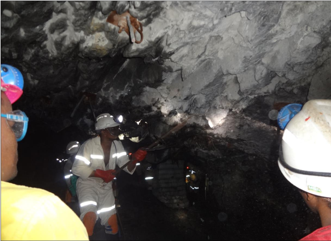
Figure 6: Blocky Pyroxenite Hanging wall
