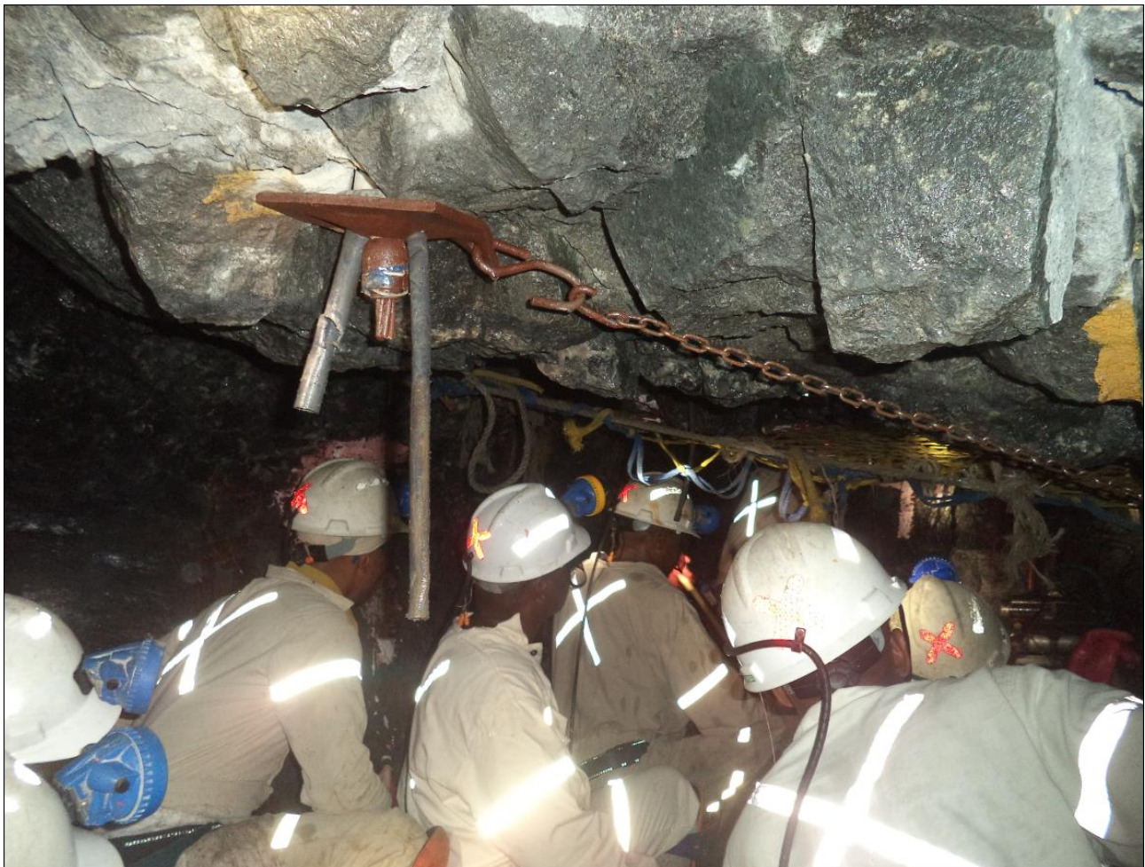
Figure 68: Blocky HW conditions
