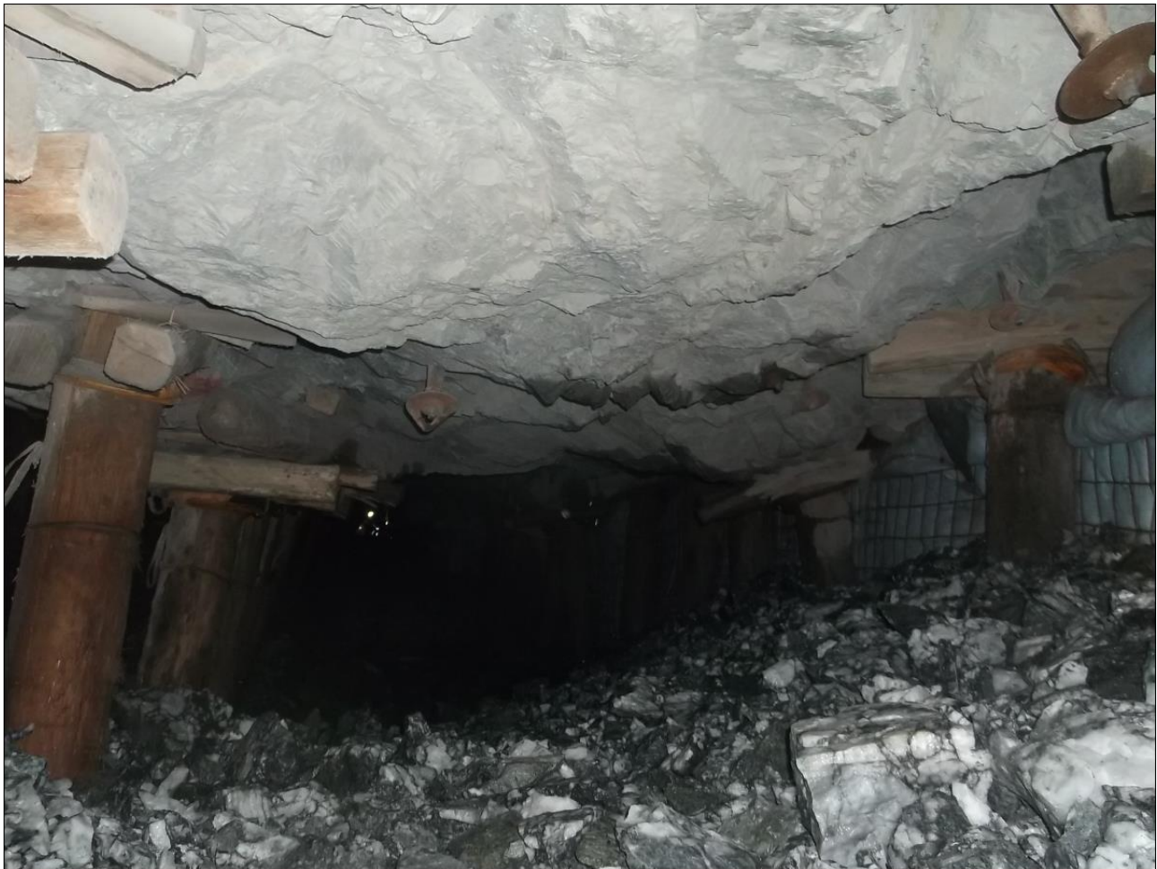
Figure 94: Lava HW with excessive accumulations of ore in-stope
