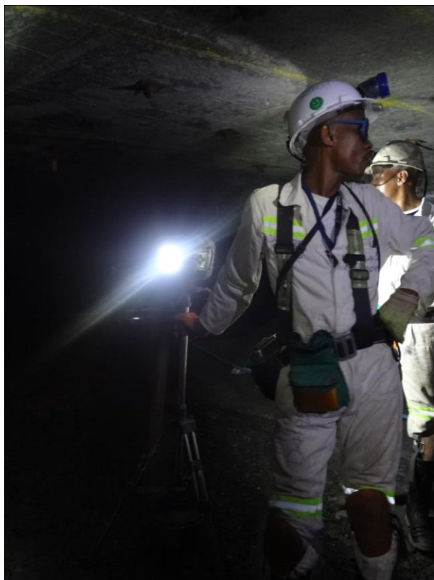
Figure 16: Use of entry examination light
