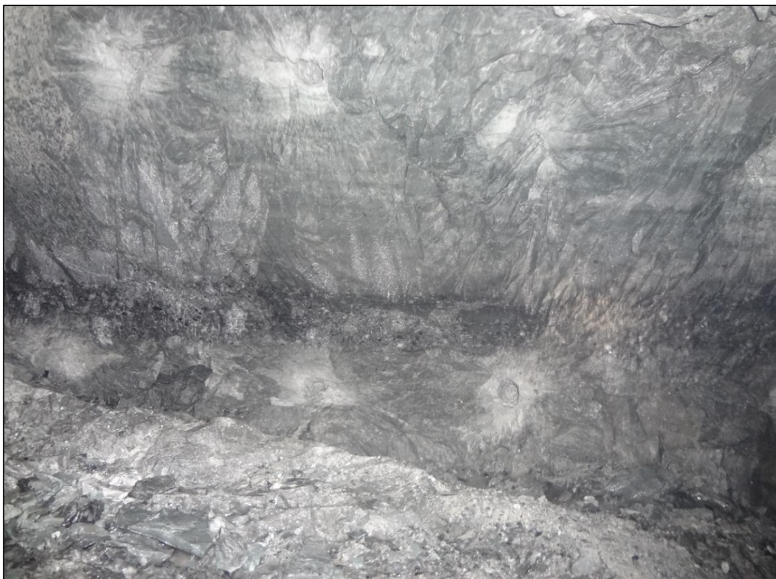
Figure 25: Multiple sockets on the face
