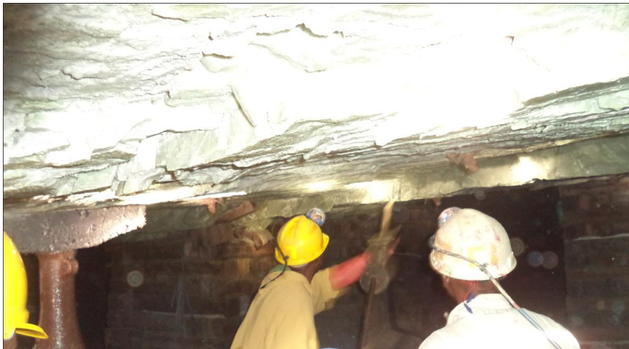
Figure 82: Laminated HW (Quartzite)
