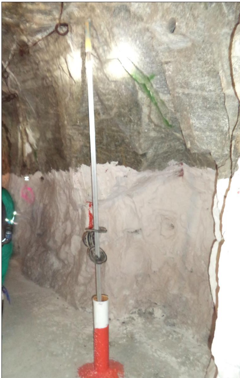
Figure 61: Pinch bars in haulage
