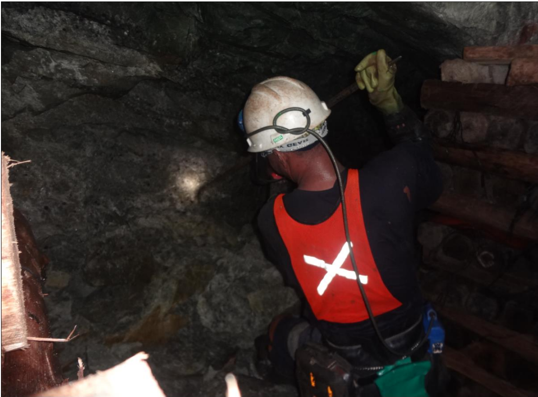
Figure 30: Positioning of barrer
