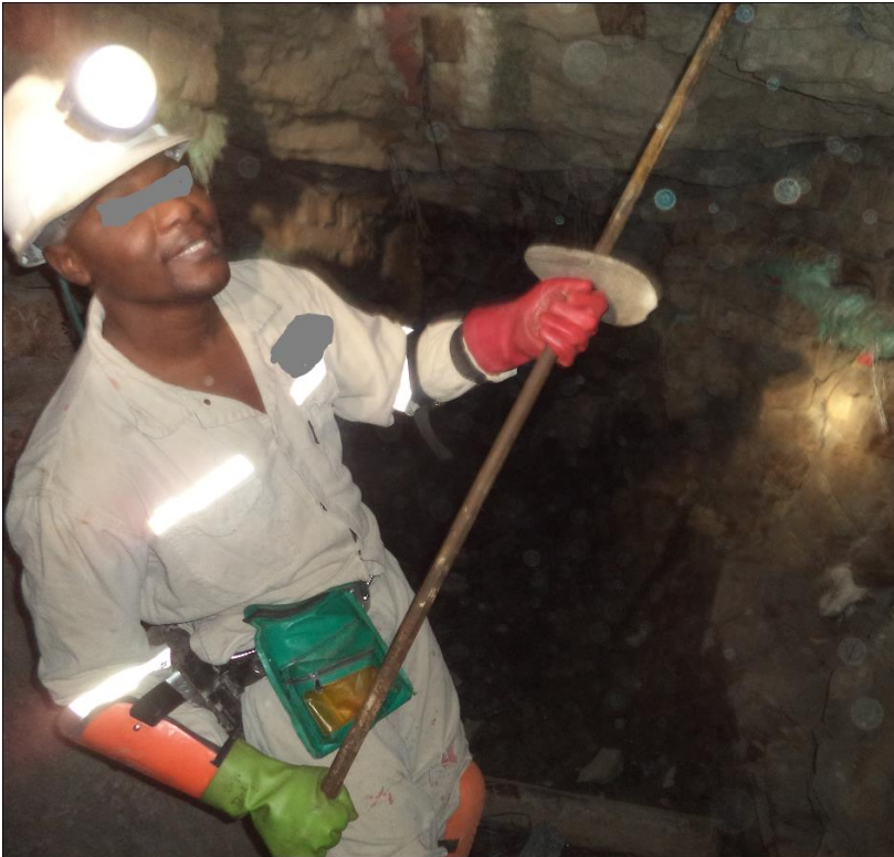
Figure 81: Barring a blocky area
