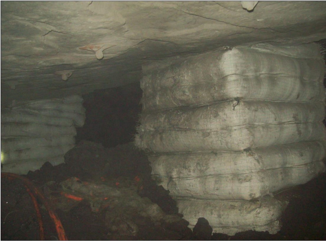
Figure 1: Smooth HW conditions
