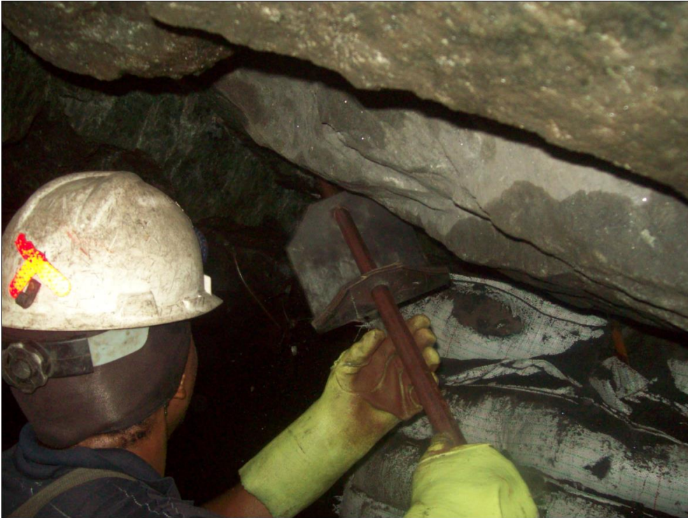
Figure 2: Barrer's hands not positioned behind/ in gasket
