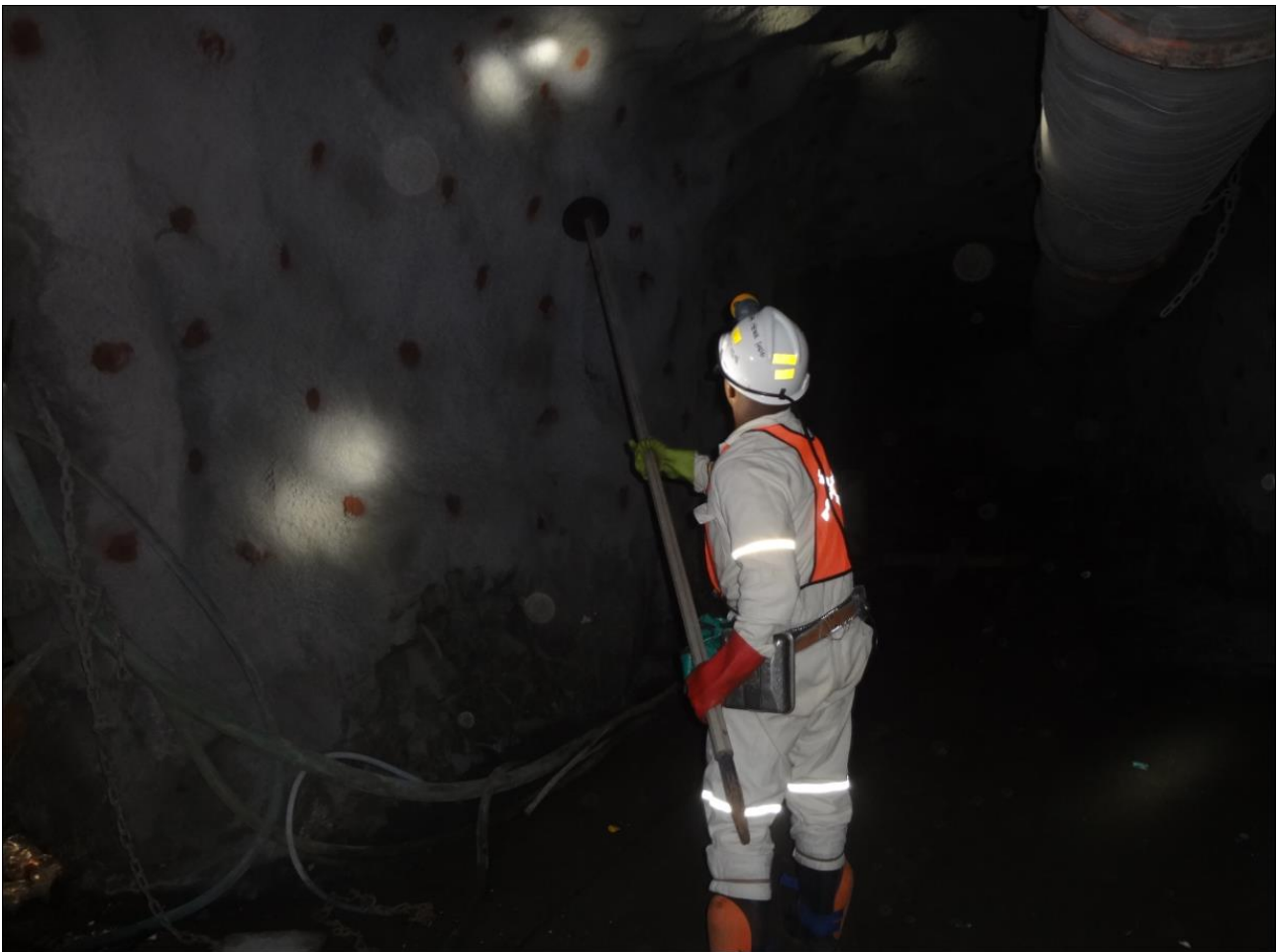
Figure 23: Inadequate barring training where trainees 'demonstrate' barring in a shotcreted area rather than actually barring
