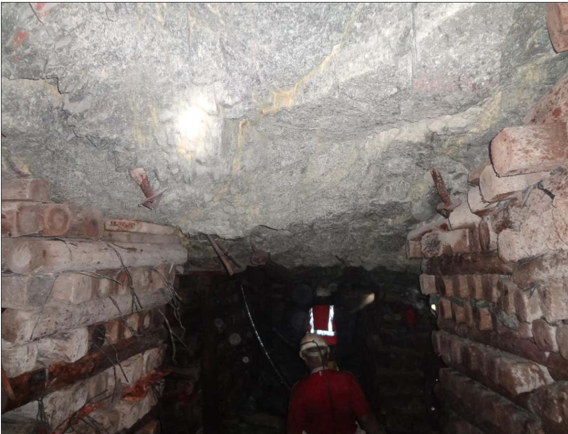
Figure 29: Fractured HW Quartzite
