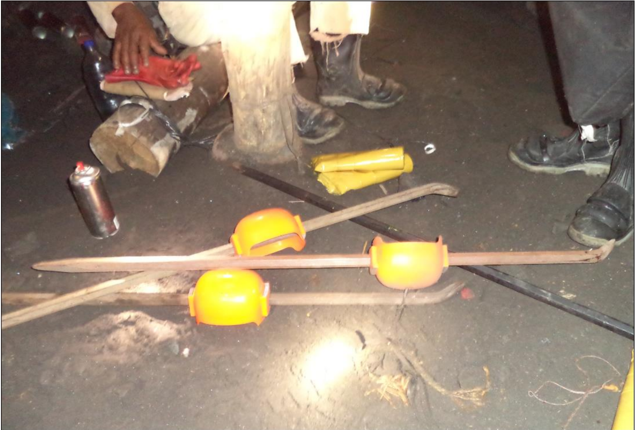
Figure 71: Orange gaskets on pinch bars
