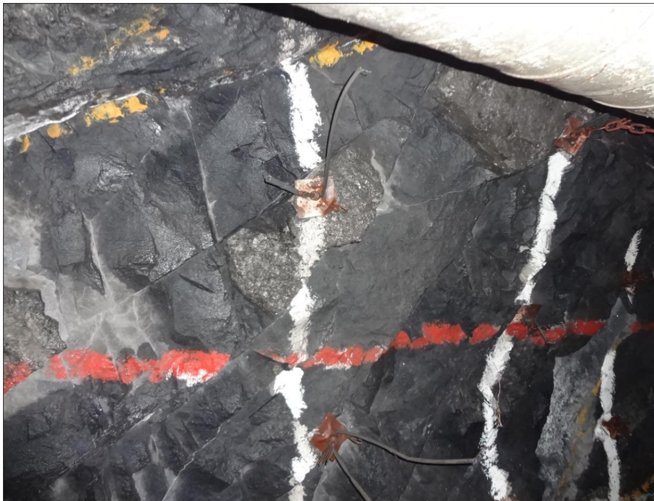
Figure 9: Jointing in Sidewall of Pyroxenite
