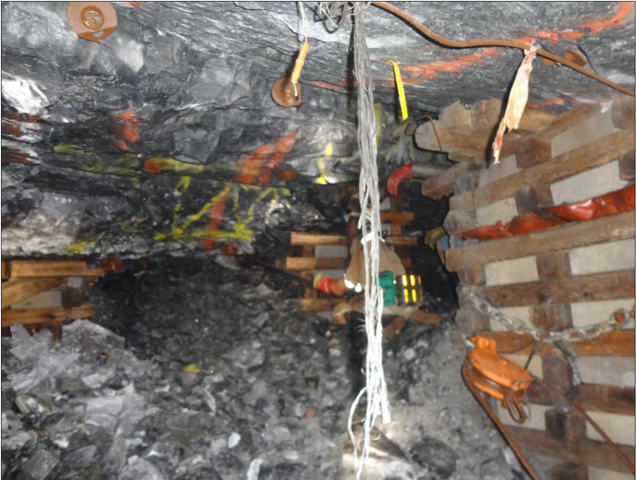
Figure 35: Fractured WAF hanging wall
