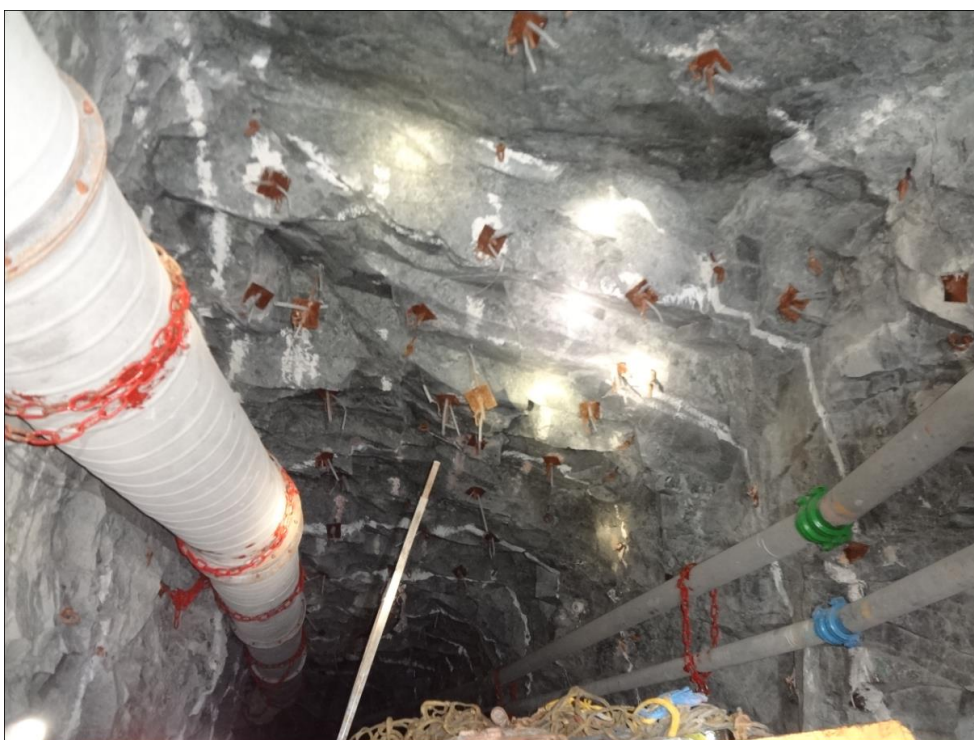
Figure 8: Support density due to faults and dykes
